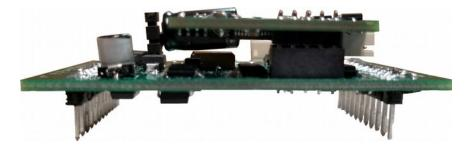
The SM18 system is a combined motor and sound decoder consisting of two stacked circuit boards. The smaller upper board handles sound while the larger lower board controls the motor, lighting and function outputs of the system.
