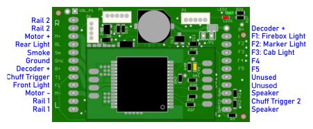
The Decoder + connection on J2 is only active on the -ST and -AR models.
