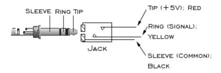
The plug is a standard 2.5mm stereo (TRS) plug. The supplied Jack is fully insulated from the mounting hole. Other 2.5mm Jacks may be substituted – but make sure that there is no ground path between the common to any of the power inputs (Terminal 1. 2 or Battery +).
