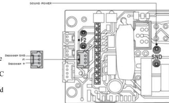
There are two pins labeled "SND" on the LGB circuit board. Slip one of the Phoenix power clips over each pin and connect to terminals 1 & 2 on the 2K2 or PB9. Since this is a DCC situation, polarity will not matter. The P5 can be powered from these pins as well.
