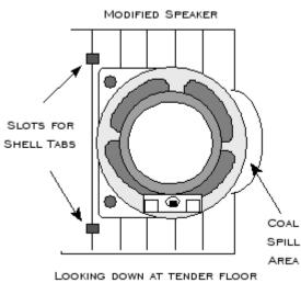
shell to fit back on the tender floor. The front edge of the speaker extends into the area where the coal spill is modeled at the forward end of the tender. Make sure that any loose pieces of the model are glued securely in place. Any extra time you spend making sure you have a good acoustic chamber is well worth the effort. Set the engine aside to allow the adhesive to set.
