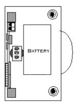
The included 3.6V battery is installed flat against the ceiling of the tender shell. The water fill hole almost touches the long edge of the battery. The second mounting pad in your kit can be used to hold the battery in place.
