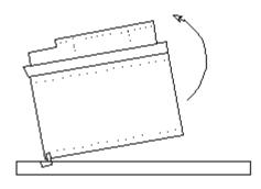
Bachmann's Operator's Manual. These openings provide access to the Philips screws that secure the tender box to the floor. Remove the two screws but do not take off the box yet. The back end of the tender box is held in place by two plastic tabs. To avoid breaking the tabs, lift the front end of the box and carefully swing it open like a hinged lid to release the holding tab and then lift off the shell.
