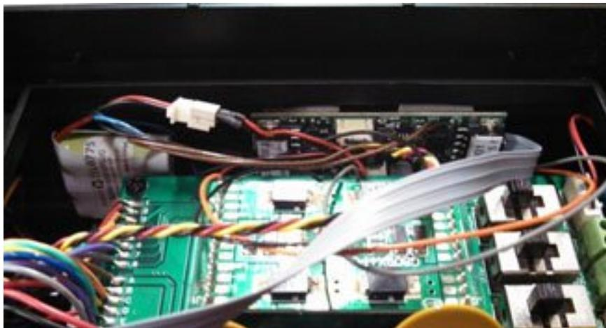
We feel one of the best locations to mount the sound board and battery is on the inside wall of the tender. Feel free to mount the board and battery where you would like. You may use the double sided foam tape squares included with the kit to mount the pieces. One square is typically enough to hold the weight of the battery or the sound board.
